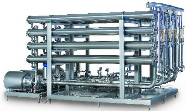
Industrial Nanofiltration System
