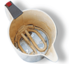
Scale deposits a kettle due to hard water
